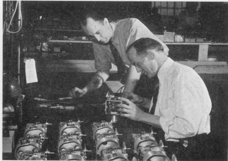
Parts assembly — L. L. Scott, a specialist in condenser assembly for 16 years, is shown working on a group of TYPE 755 Condensers, under the direction of H. J. Comrie, foreman.
